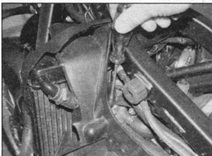
4.1 Remove the heat shield
