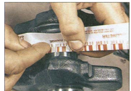
3.16 Measuring the width of the crushed Plastigauge
