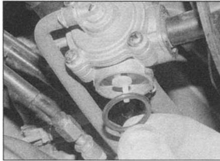
10.4a Install the strainer and fit a new O-ring ...
