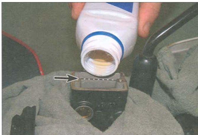
3 Top up with fluid of the recommended type until the level is up to the ridge along the inside of the front wall of the reservoir (arrowed). Do not overfill.
