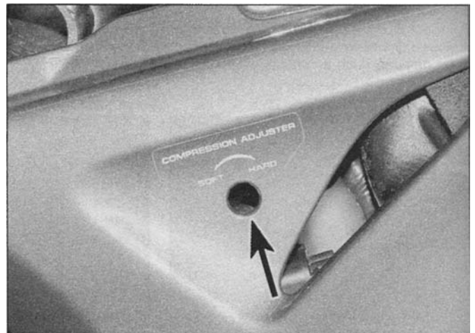
13.6 On XL650V models, adjust compression damping via the aperture (arrowed)
