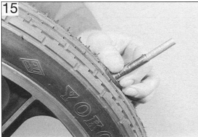
Checking the tyre tread depth
