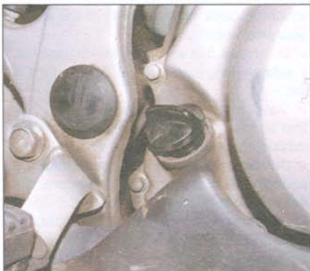
3 Insert the clean dipstick back into the engine, allowing it to rest on the bottom thread of the cap - do not screw it in.
