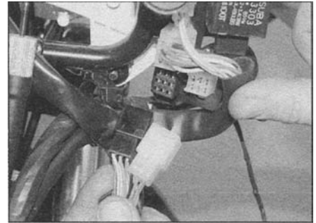
15.3b Instrument cluster wiring connectors - XL650V
