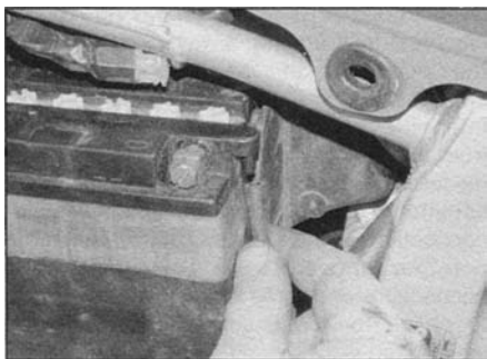
3.3c Disconnect the breather tube
