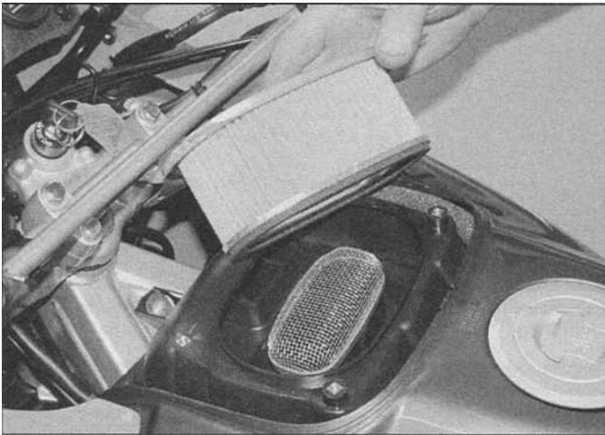
8.3c ... and withdraw the filter
