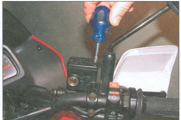
2 If the level is below the LOWER line, undo the two reservoir cover screws and remove the cover, diaphragm plate and diaphragm.
