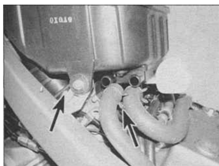
4.10 Slacken the clamp screws (arrowed)
