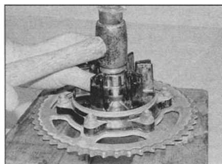
15.27 ... then drive out the bearing
