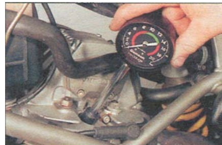
3.20 Using a rubber-cone type cylinder compression gauge
