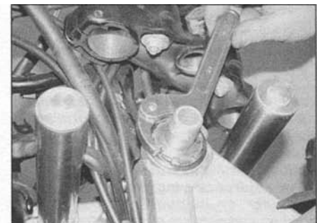
23.10 Adjust the bearings as described using either a C-spanner or a drift, or one of the special tools described
