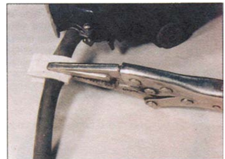
9.4 ... or thick card and self-locking grips
