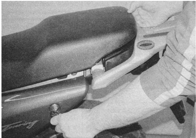
2.3a Unlock the seat, lift it up at the rear and draw it back...
