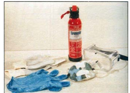
1.6 A fire extinguisher, goggles, mask and protective gloves should be at hand in the workshop
