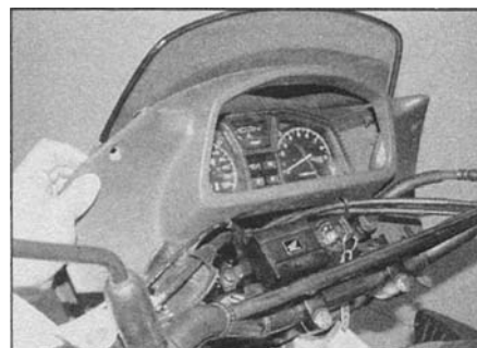
4.2 Undo the four screws and remove the panel
