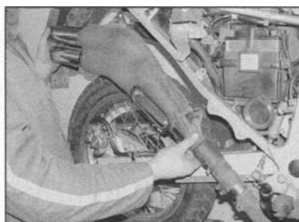
13.2d ... and remove the silencer
