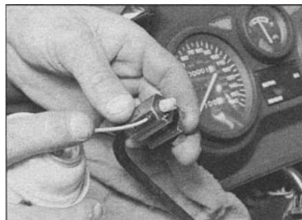
12.3a Lubricating a cable with a pressure lubricator. Make sure the tool seals around the inner cable
