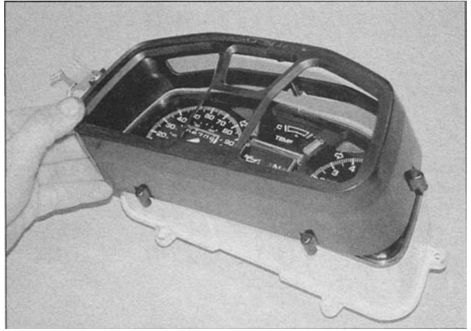
16.4b ... then remove the outer cover ...
