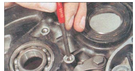
2.30 ... break off the tang when complete
