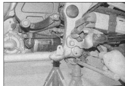
13.6b ... with a socket extension is the easiest...
