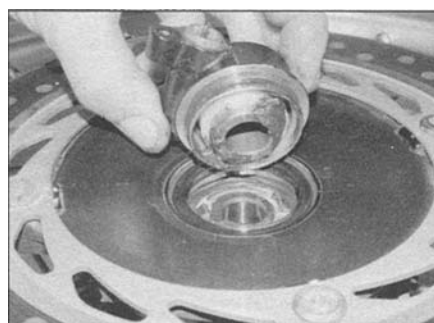
13.6a Remove the speedometer drive housing ...
