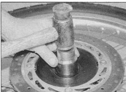
15.11b ... or use a socket to drive it in if necessary
