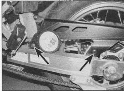
14.3b Chainguard bolts (arrowed) • XRV750
