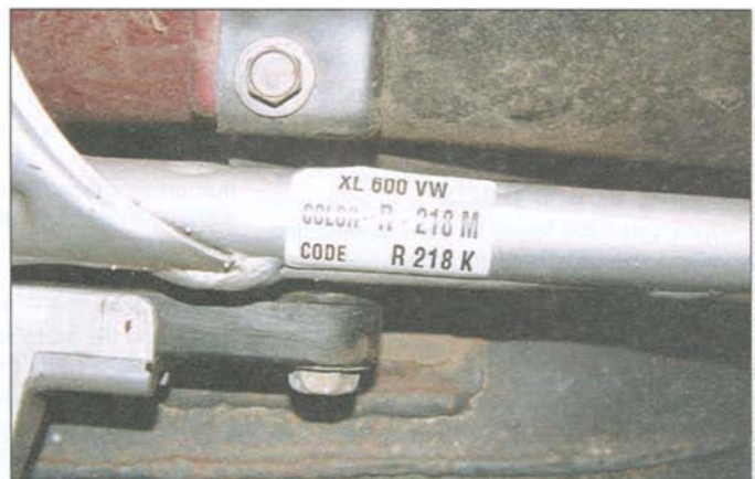
The colour code label is on the rear subframe
