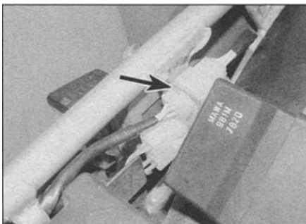
32.1a Alternator wiring connector (arrowed) - XL600V
