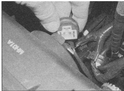
7.2b Disconnect the wiring connector - XL650V
