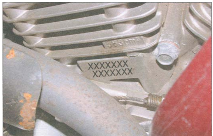
The engine number is stamped into the Crankcase on the right-hand side of the engine
