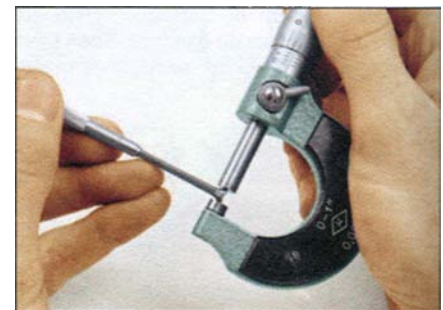
3.10 ... then measure the gauge with a micrometer
