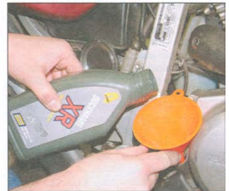
5 If the level is below the lower mark, top the engine up with the recommended grade and type of oil, to bring the level up to the upper mark on the dipstick.
