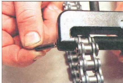
8.2 ... withdraw the pin, remove the tool...
