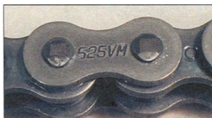
8.10 Typical chain size and type marking
