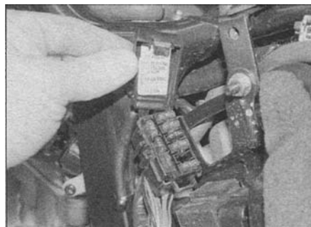
5.3e ... to access the fuses
