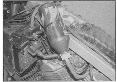
17.9 One way of setting up an auxiliary fuel supply
