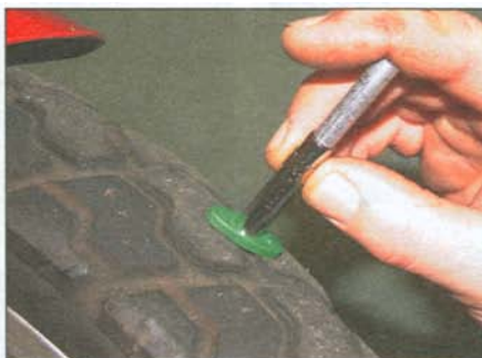
2 Measure tread depth at the centre of the tyre using a depth gauge.
