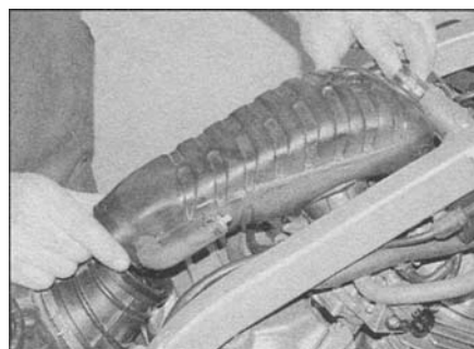
4.2d Lift the duct housing up off the carburettors
