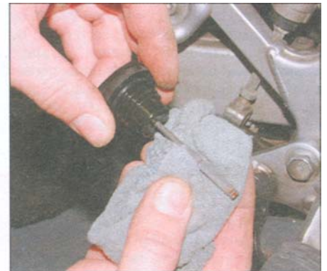
2 Using a clean rag or paper towel, wipe off all the oil from the dipstick.
