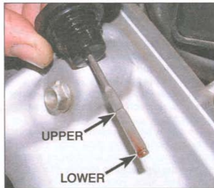
4 Remove the dipstick and observe the level of the oil, which should be somewhere in between the upper and lower level marks (arrowed).
