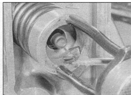
14.5c Remove the collets as described
