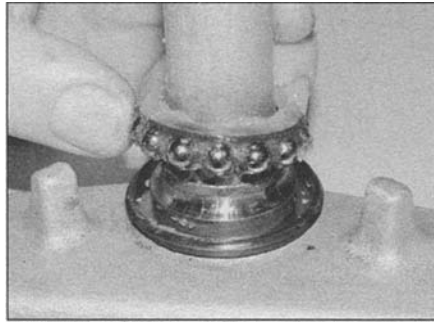
9.6c Remove the lower bearing from the steering stem
