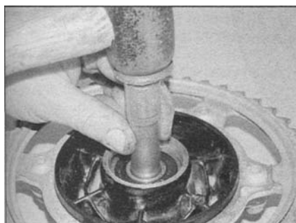
15.26 Drive out the spacer...
