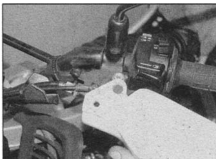
12.3c ... and remove the handguard
