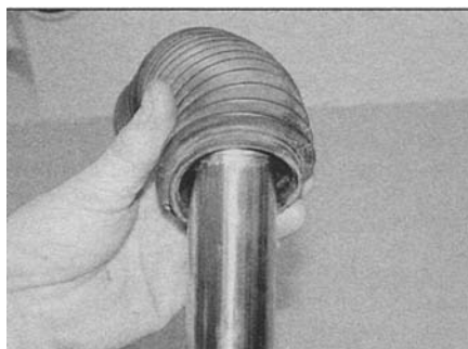
8.2 Remove the gaiter
