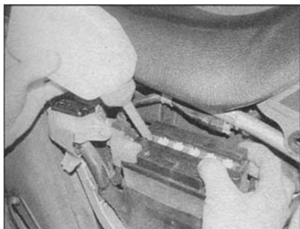
6.3b ... and top up the cell with distilled water
