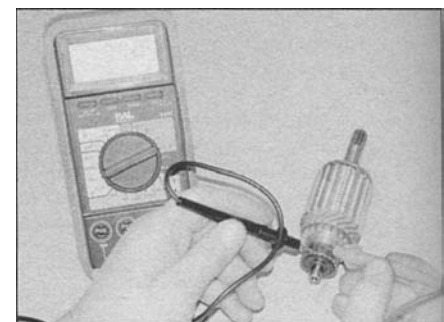
29.11 Continuity should exist between the commutator bars
