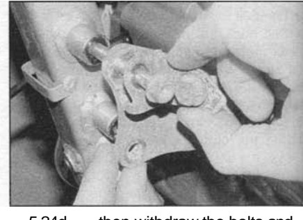
5.24d ... then withdraw the bolts and remove the left-hand piece, noting how all components fit
