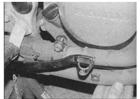
13.3e ... and remove the pipe
