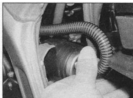
11.10a On XR750 models displace the fuel pump from its mount
