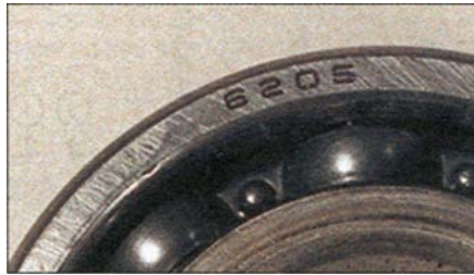
5.16 Typical bearing marking
