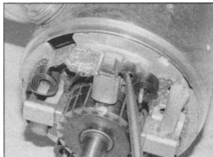
29.17 Locate the spring ends onto the brushes
