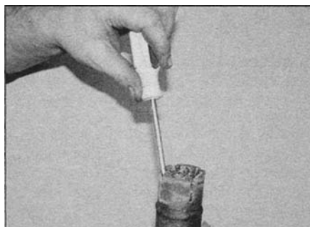
13.7a Dig out the old sealing ring ...
