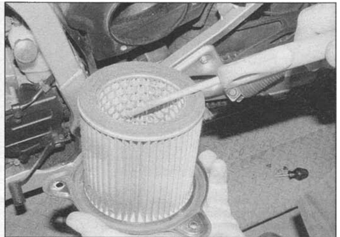
8.4 Direct the air in the opposite direction of normal flow
