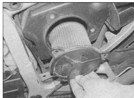
8.1b ... and withdraw the filter
