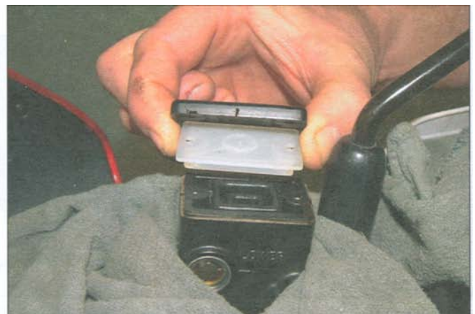
4 Ensure that the diaphragm is correctly seated before installing the plate and cover.
