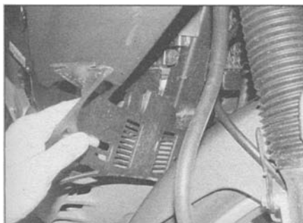
5.19b ... and remove the stone guard
