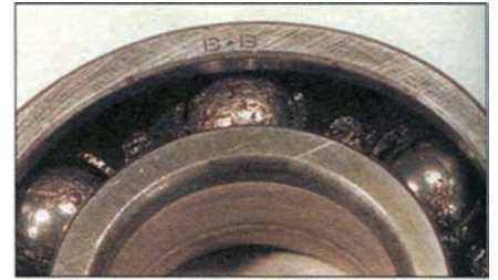
5.18 Example of ball journal bearing with damaged balls and cages
