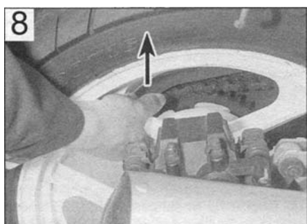
Checking for rear suspension linkage play
