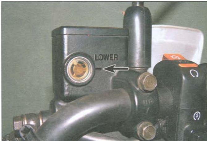
1 The front brake fluid level, visible through the window in the reservoir body, must be above the LOWER level line (arrowed).
