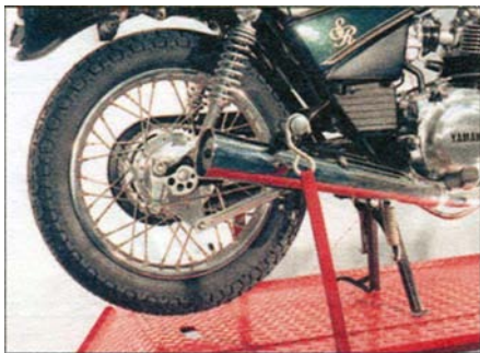
1.2 Tie-downs are used around the passenger footrests to secure the bike
