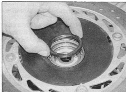
15.11a Fit the grease seal and press it into place...
