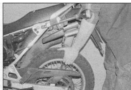
22.7b Checking for play in the rear shock mountings and suspension linkage bearings
