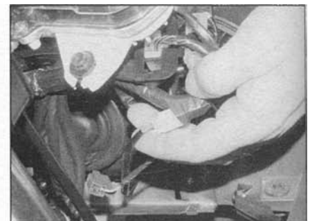
5.8d ... and the sidelight wiring connector
