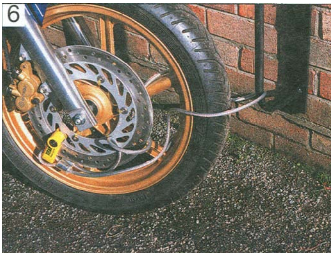
A disc lock combined with a security cable provides additional protection
