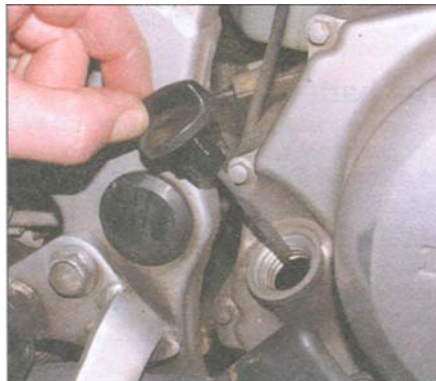
1 Unscrew the oil filler cap from the right-hand side Crankcase cover. The dipstick is integral with the oil filler cap, and is used to check the engine oil level.
