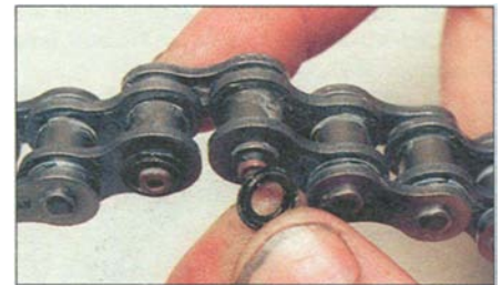
8.5 ... install the O-rings over the pin ends ...
