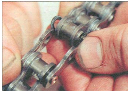
8.3 ... and separate the chain link
