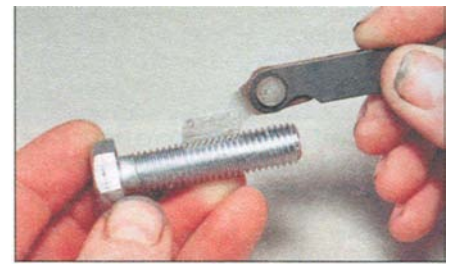
2.12 Using a thread gauge to measure pitch
