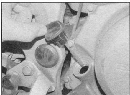
13.3 Unscrew the oil filler cap to act as a vent...
