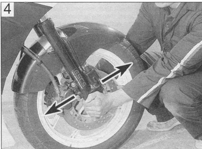
Checking the steering head bearings for freeplay
