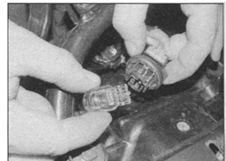
9.3b ... and the bulb from the holder (arrow)
