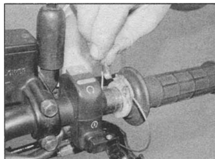
11.4d ... then detach the cable ends from the pulley ...
