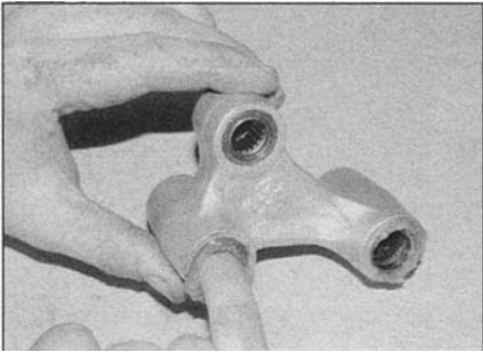
12.11 Smear the bearings with grease
