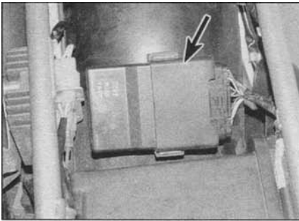
5.3a Ignition control unit (arrowed) - XL600V
