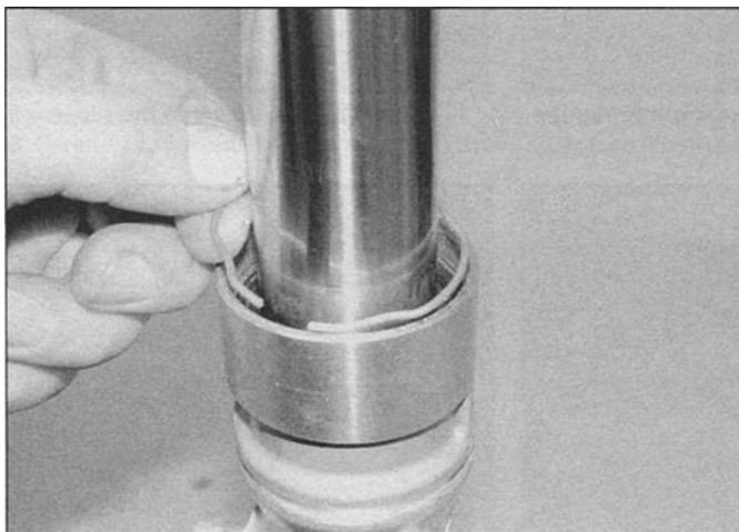
8.24 Install the retaining clip ...
