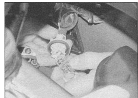
12.4d ... then pull the bulb from the holder
