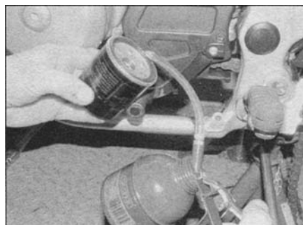
13.7a Smear clean oil onto the seal...
