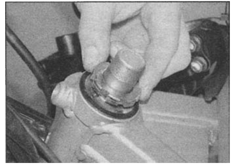
9.4a Unscrew and remove the adjuster nut...
