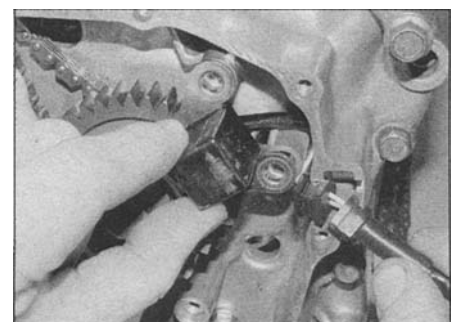
4.17b ... then free the wiring grommet and remove the coil - XL single coil model shown
