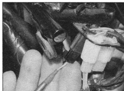
4.10d ... and the sidelight wiring connector
