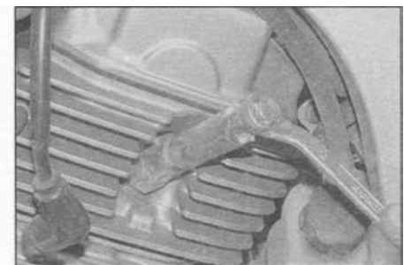
5.5b If you are using the Honda tool, locate it onto the plug and use a ring spanner to turn it
