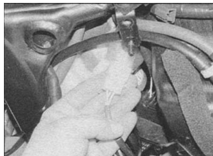
32.1b Alternator wiring connector - XL650V
