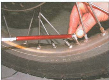
1 Remove the dust cap from the valve and check the tyre pressures when cold . Do not forget to fit the cap after checking the pressure.
