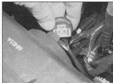
5.8c ... and disconnect the headlight wiring connector ...
