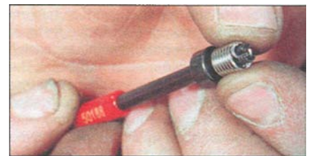
2.28 ... fit insert on the installing tool...
