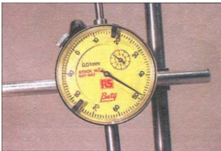
3.17 Dial gauge reading of 1.48 mm
