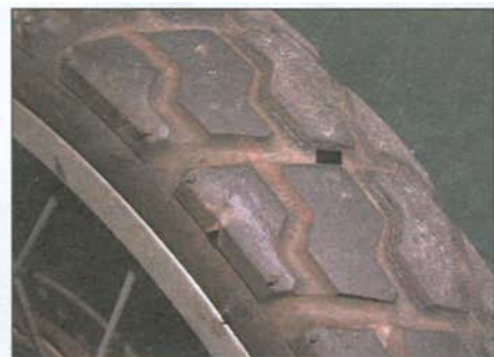
3 Tyre tread wear indicator bar and its location marking (usually either an arrow, a triangle or the letters TWI) on the sidewall.
