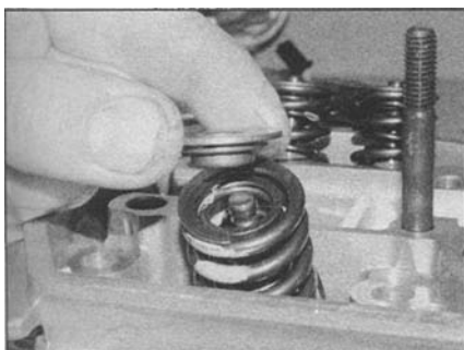
14.28c ... then fit the spring retainer
