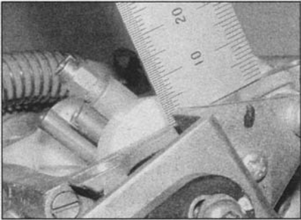
10.8 Measuring the float height
