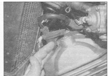
5.2b Front cylinder - left-hand plug
