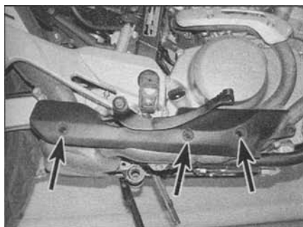
13.1d The shield on the XL650V is secured by three bolts (arrowed)
