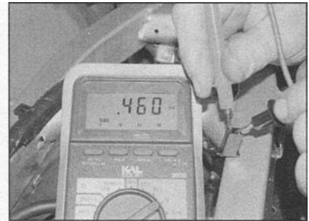
4.6 Measuring pulse generator coil resistance
